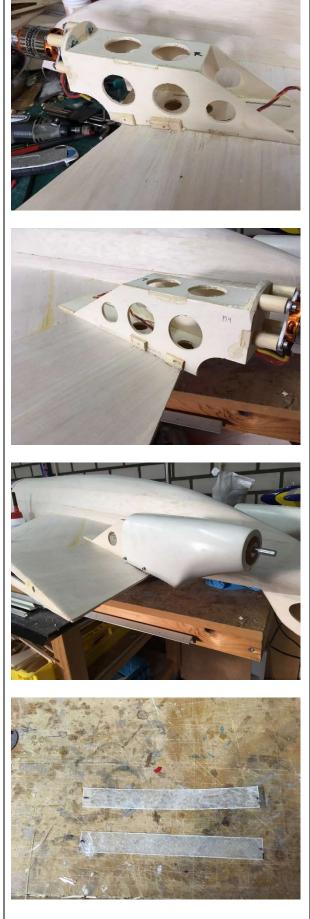
Glue 2 M3 impact nuts in the engine cowl for fixing the front and back of the engine cowls together.
