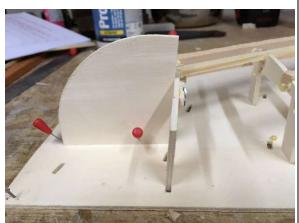
Glue WC-7 on top of ribs WC-1 till WC-6. Glue leading-edge WC-10 on the front side of ribs WC-1 till WC-6.
