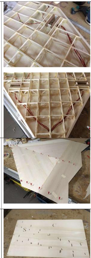
The leading-edge side of ribs WC-1 till WC-6 have to be sanded in a bit of an angle. This also must be done for the cut-outs in WC-7 till WC-10.
