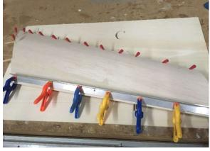
Take the front wing out of the template and put pencil marks on the topside for the control surfaces. To show the contours of the control surfaces, push a long needle through the sheeting between "S12 and S13". The needle has to go from the underside of the wing through the sheeting of the topside.
