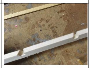
Glue part "S12" onto ribs "S1" to "S8". Glue part "S13" onto ribs "S3a" to "S8".
