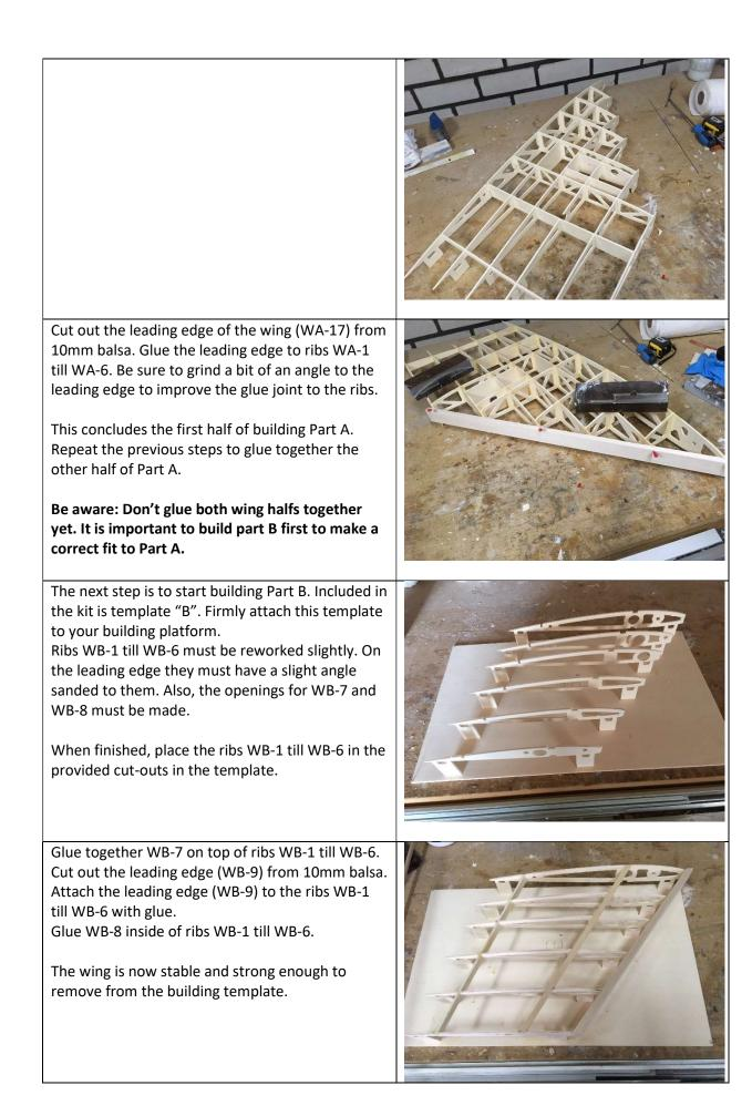
It is very important to make the correct fit between Part A and Part B.
