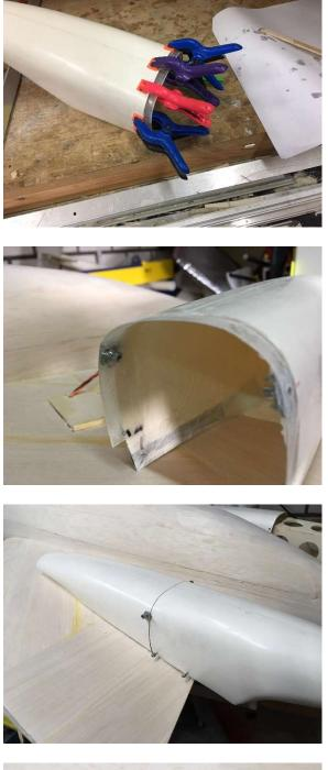
Glue a piece of wood with a notch on wing part A. The front of the engine cowl will be clamped under this.
