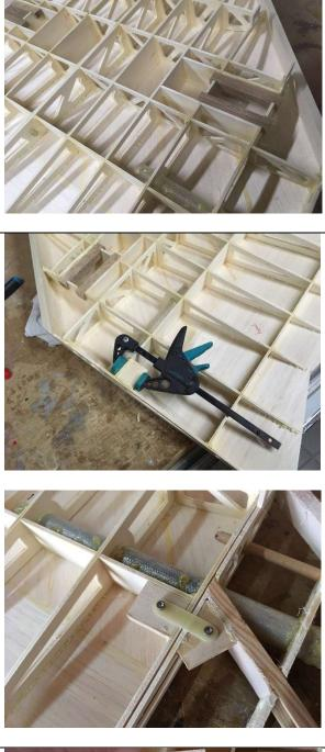
Cut out an extra reinforcement piece from some 1,5mm leftover balsa. This reinforcement has to be placed between ribs WA-3, WA-4 and side-ribs WA-11, WA-12. Glue to the top-side of the sheeting.
