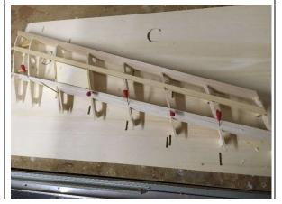
Before sheeting the front wing with wood the parts "S11, S12 and S13" have to be scuffed to fit the correct size.
