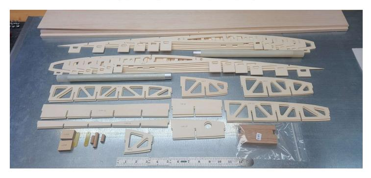
**Builders Note** – If you plan to install the WA-20 8mm hardwood dowel in the nose of the Main Wing, now would be the time to cut 8mm notches in both WA-1 ribs for the dowel to fit into.
