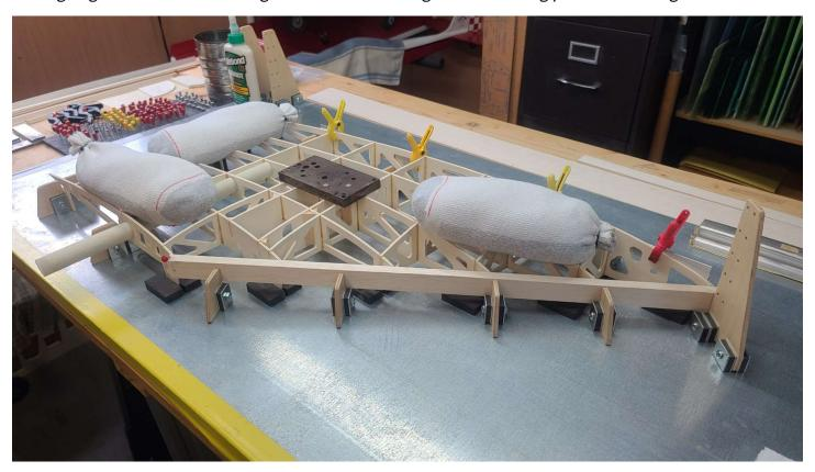
After going through all the same steps again to build the left inboard-wing panel, I pulled that panel from the mag jig and as you can see in the image below, we now have both panels needed for the Main Wing inboard section. Next up is to start the build of a Main Wing mid-wing panel.
