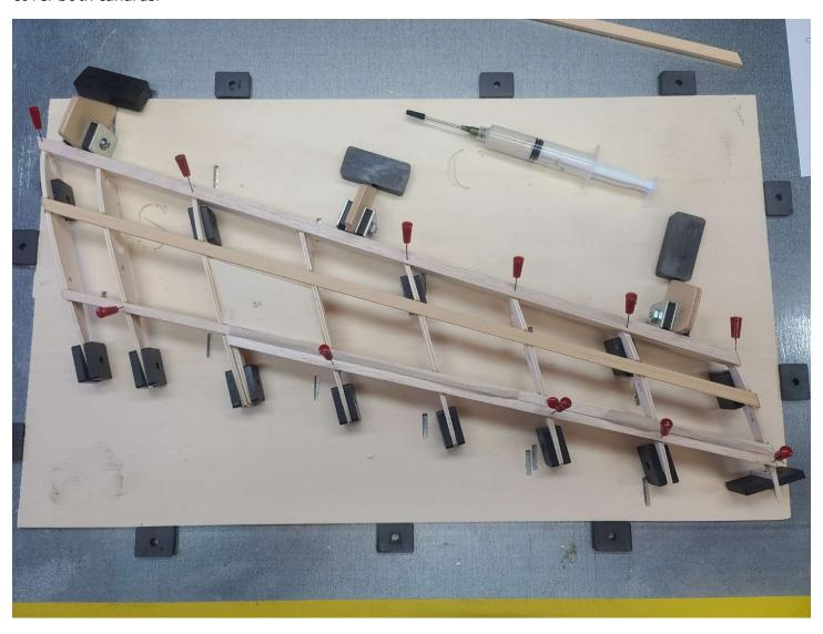
After a complete sanding of the canard to the final top airfoil profile of the ribs, the 1.5mm balsa sheeting was applied. The image below shows the gluing of this top balsa sheeting on the right canard. I use old socks filled with lead shot to apply weight evenly over the surface while the glue dries. These work great!
