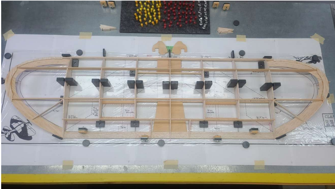
Figure 5 – Modified Top Wing Full-Up Dry Fit Check on Magnetic Build Board
