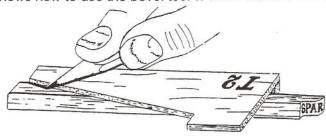
C) Sketch C shows the end of a spar being cut as marked. NOTE: Some spars need to be cut at an angle. The dotted line shows the angled bevel, the solid straight line shows a square bevel.
