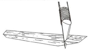
Now pin and glue the Leading Edge assembly into place on the plans. The center wing ribs have slots in them to accept tabs on the pilot shelf, throttle servo tray, and rib spacer. These should all be in place between the center ribs before the ribs are pinned in place on top of 1/16" balsa shims (the shims are used because of the cap strips). NOTE: The throttle servo tray should be assembled and the throttle servo should be test-fitted before installing the tray.
