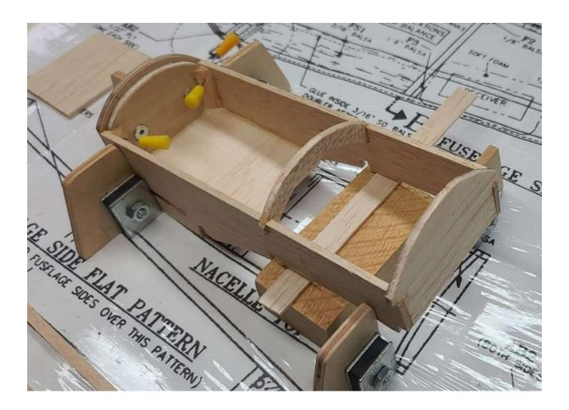
How about we start the fuselage for this scratch build! Again, using the templates from sheet 3 of the plans, cut out and shape the parts needed for the left fuselage side from 3/16-inch balsa sheet. Then, as shown in the picture below, the left fuselage side is built directly over the <u>fuselage side flat pattern</u> on sheet 1 of the plan.
