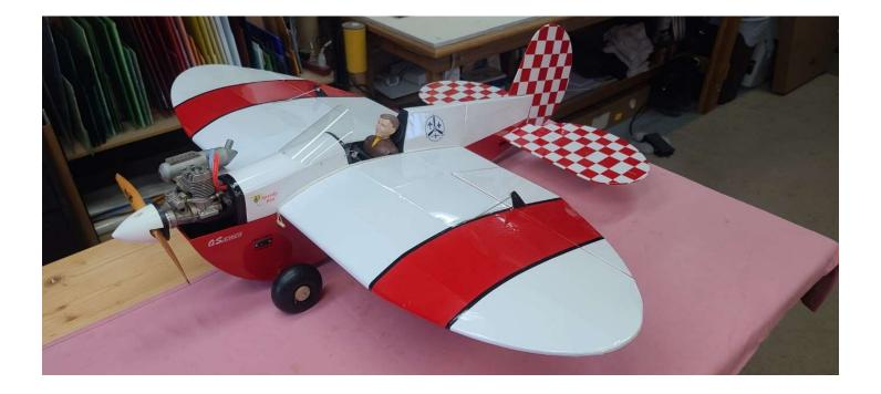
Overall, this has been an interesting scratch build. I learn something new from each one. One item I think I'm going to address is the landing gear mounts. Using rubber bands doesn't provide a very stable gear and the model wants to rock to one side or the other. The Clancy assembly instructions have an option using RC racer spring shocks and they will be simple to add even with the build completed.
