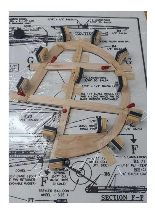
The horizontal stabilizer and elevator are a very simple build using 1/8-inch balsa sheets. I'm not building my Speedy Bee with the removal tail option, so this eliminates the two holes along the front edge of the horizontal stabilizer. Last item for this assembly is to cut out the six hinge slots and sand everything to shape.
