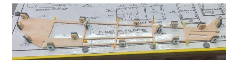
By using the mag fixtures, I can position all the parts together to check twice for proper fit. Prior to gluing, use the parts from the left fuselage side to cut and shape all the parts that will be required for the right fuselage side (minus the power switch mounting holes in C1). With that done, glue up all the parts for the left fuselage side.
