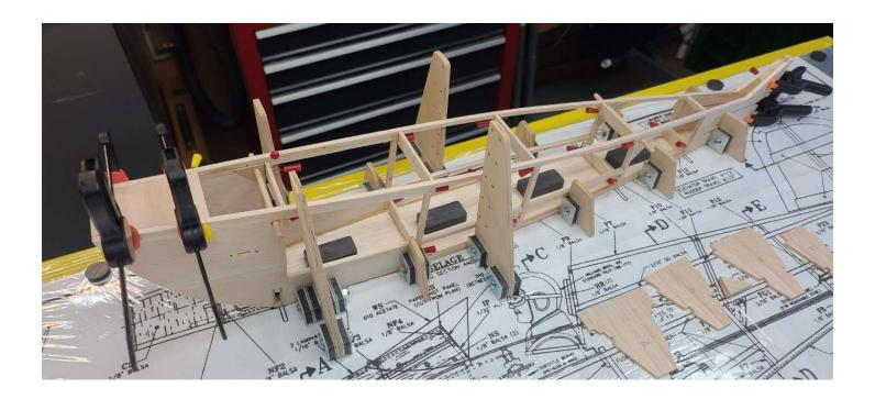
When everything has dried, the fuselage gets removed from the mag board so I can sheet the front using two layers of 1/16-inch balsa sheeting. Then I sand all the fuselage sides down using 100 grit on my Duo-Bro sanding bar so everything is nice and smooth.
