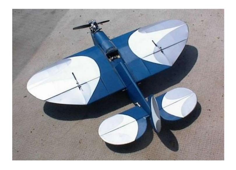
The Speedy Bee is light enough to fly with glow engines as small as the Cox .09, and strong enough to handle larger engines up to .25 sport two-cycles or up to .30 four-cycles. It will climb at an angle of about 75 to 80 degrees on a sport .15 and have a take-off roll measured in inches rather than feet. With larger engines it will probably have vertical capabilities.
