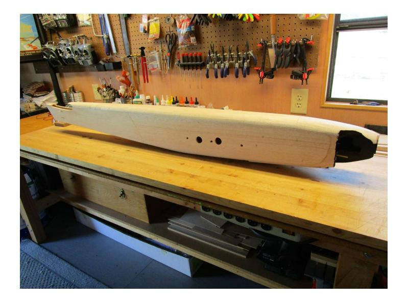
This picture shows the fuselage fully assembled with engine cut-out and the outside sanded down to get the required overall shape needed. A large hatch is placed in the bottom of the fuselage to obtain access to all the radio gear, servos, fuel tank, receiver battery, and wing mounting screws.
