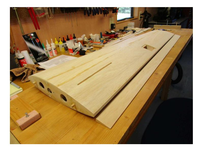
With this complete, accomplish the same steps for the right wing. Install the balsa block wing tips and sand to shape. Sand the entire surface using 220 grit to prep the wings for covering. Let's move on to the tail surfaces.
