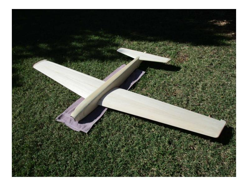
Initial test fit of the wings and horizontal stab are made to check over fitting prior to covering. I also accomplished a total up fit check with engine, MLG, NLG, and vertical tail installed to establish the amount of weight I need to put in a wingtip for proper lateral balancing.
