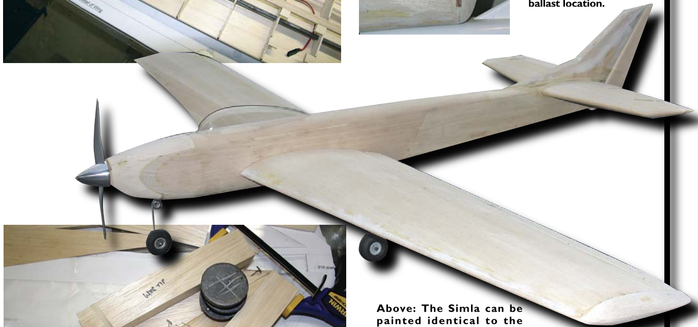
Near left: The overall model should be laterally balanced. A small plate has been added to seal the ballast location.
