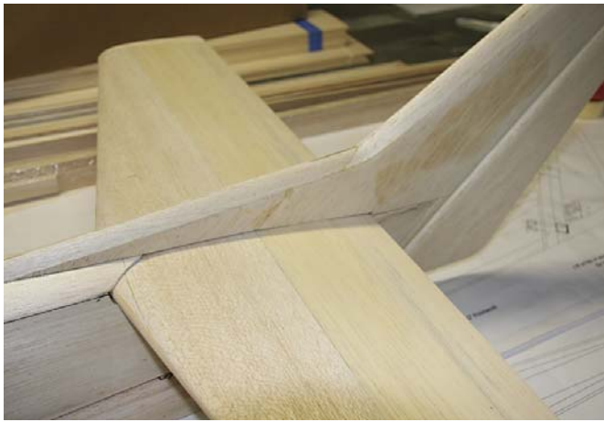
The stabilizer/elevator is built as a whole and fully sheeted before cutting away the elevator and adding the stabilizer TE and the elevator LE.
