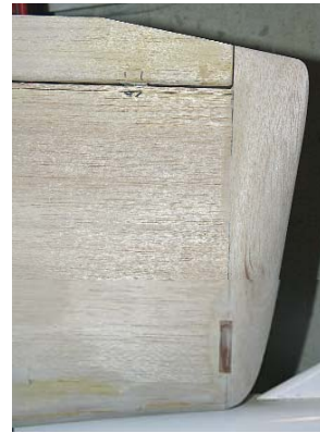
Far left: The top balsa sheeting is added, and then the build tabs can be removed and sheeting the lower surface can proceed. The modern wing-tube mounting system is a welcome change from the original.
