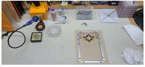
Once you are good with the fit of a glass piece, move over to the foiling station (see below) to apply copper foil to the edges on each piece of stained glass, and then place them back over the pattern at your assembly area (image above). Note – I
