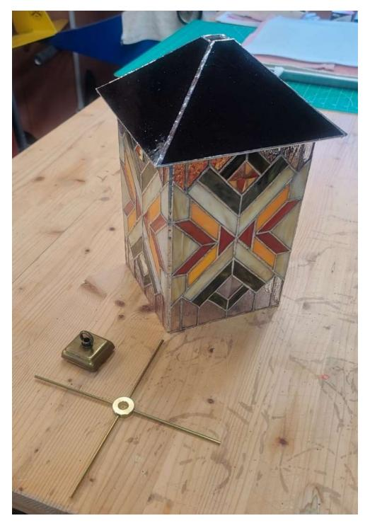
I used black patina to color the solder joints on the black top, and then assembled all the lamp hardware and wiring for the LED light. With everything assembled, I finished the project by mounting the transformer on the wall inside my workshop, and then the lantern outside above the entryway. The final image below shows the finished lamp outside in a light misty rain. I think it turned out real nice and it will look great at night.
