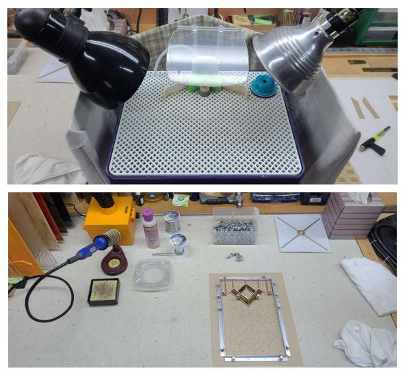
Once you are good with the fit of a glass piece, move over to the foiling station (see below) to apply copper foil to the edges on each piece of stained glass, and then place them back over the pattern at your assembly area (image above). Note -1
