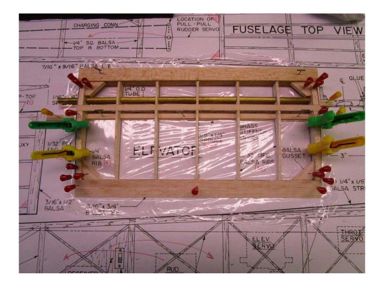
As can be seen above, I inserted the brass tube during the build to help align all the elevator ribs. As with the rudder, sanding must be done to shape the elevators to the final shape as shown on the plans. I used basswood for the elevator spars versus spruce as called out on the plans.
