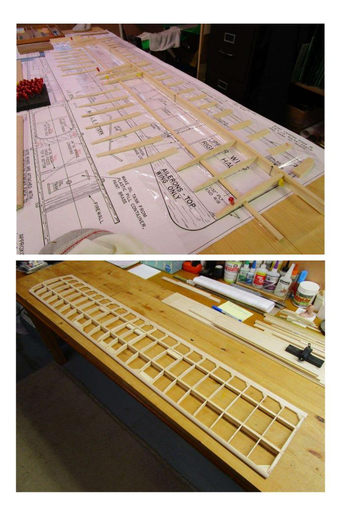
Below is the top wing in work over the plans. Similar under-camber airfoil and spar construction as the bottom wing except for the two ailerons, which will be controlled by a single center mounted servo using flexible Gold-N-Cables running inside the wing. The top wing has a total of <u>146 individual cut pieces</u>.
