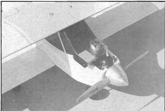
TOP ROW, LEFT: 1/2" sq. maple wing mounting blocks being glued into the fuselage. Clamps hold things together until epoxy sets. TOP ROW, RIGHT: Fuselage assembly ready to cover. ABOVE: Lower wing removed to show radio installation and rear portion of 8 oz. tank. ABOVE, LEFT: Aileron servo installed in the lower wing. Clevis on the ends of the connecting rods allows quick and easy hook-up. RIGHT: Aileron connecting rods attached to plywood horns epoxied to the ailerons. Four ailerons allow this biplane to roll like a pattern ship. BELOW, LEFT: K & B .40 with Du-Bro muffler installed gives good power but not excessive speed. Wings mount with two nylon screws. BELOW RIGHT: Double Trouble coming at you. Trike gear and absence of cabanes or struts is simple and practical.
