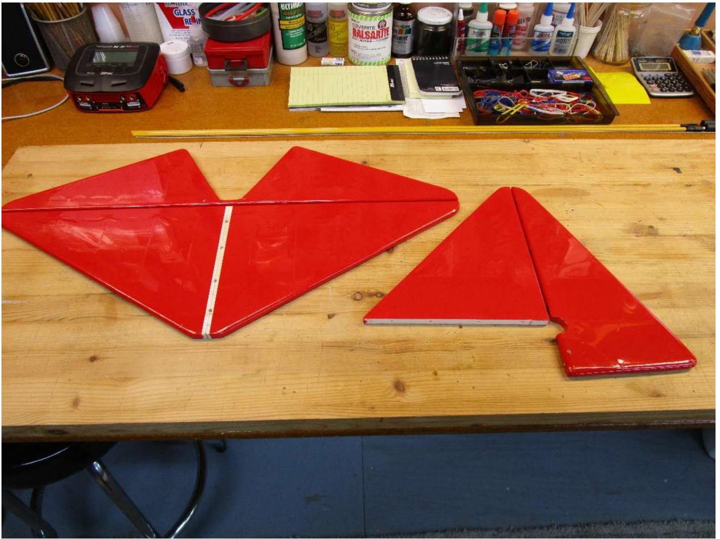
The tail feathers are covered with red Ultracoat, and Robart pin hinges are temporarily installed. Hardwood dowels will be used to strengthen the matting between the vertical stab, horizontal stab, and the fuselage.
