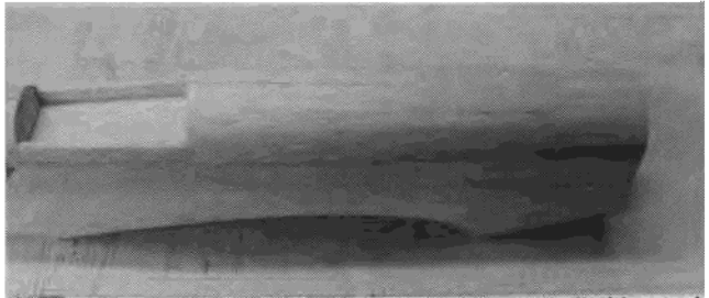
Glue on the top front 1/16" sheeting. Add the cockpit sides and shape.
