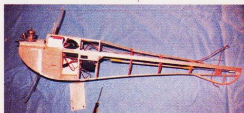
Loads of detail here. The aerial is threaded through carefully to avoid snagging, exiting centrally at the fin. The lower servo allows a straight operation of the elevator, while the upper closed loop system is just visible. Finally the battery hatch construction can be appreciated.
