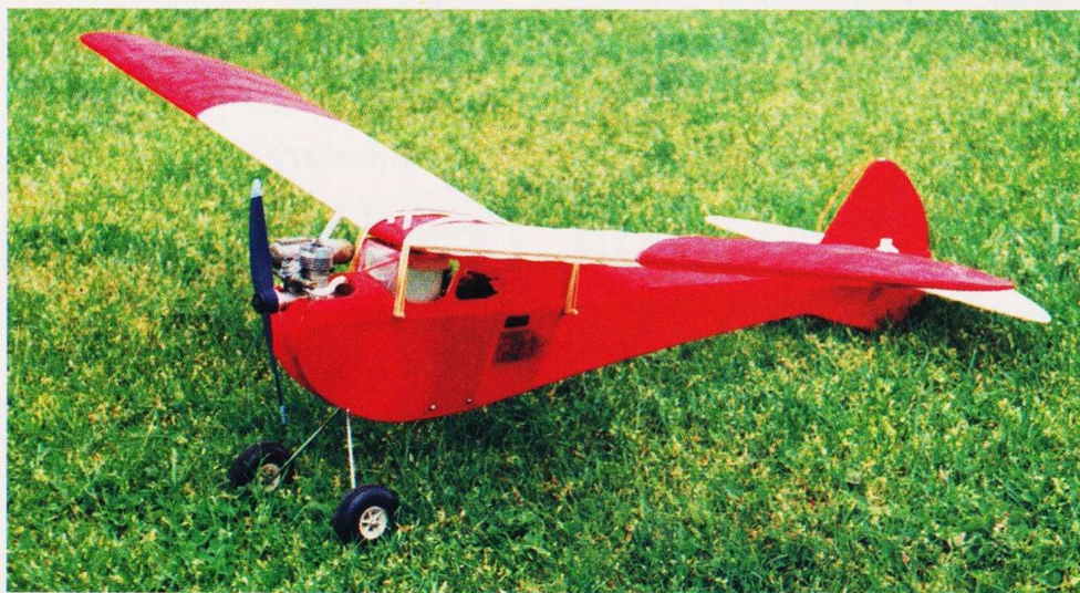
The Diamond Demon, Starspan covering, OS 10 engine, Radio Active prop, Ripmax battery, and so much more!
