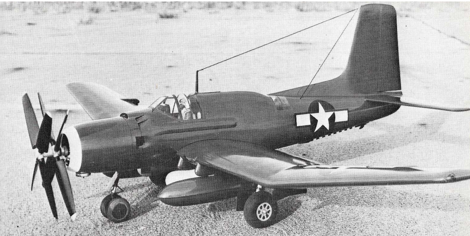
The aerial is simulated with elastic cord, allowing the Skypirate to be turned over for starting the inverted engine.
