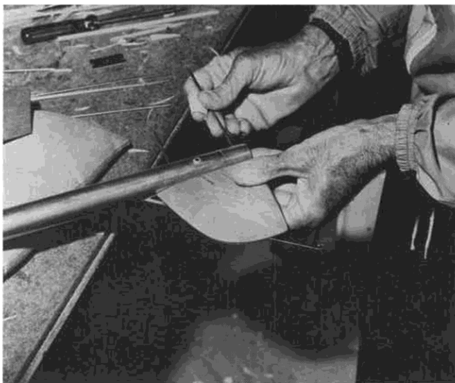
Tail surfaces are entirely demountable. These wires hold the upper fin in place. Elevator horn is in the sub-fin.
