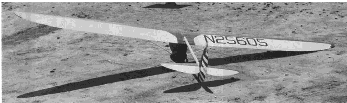
The practically non-existent dihedral presents no problems, since the model has rudder and aileron controls. By coupling them electronically, the turns come out beautifully coordinated.
