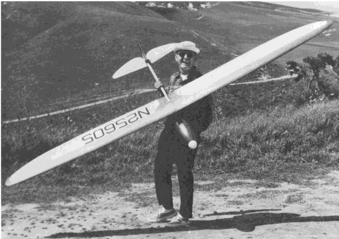
Taken the day of the first test flights, this photo proves that Bob was fairly pleased with the results. Actually, the only change required was to move the balance point aft a half inch. Ship has over 1400 square inches of wing area.
