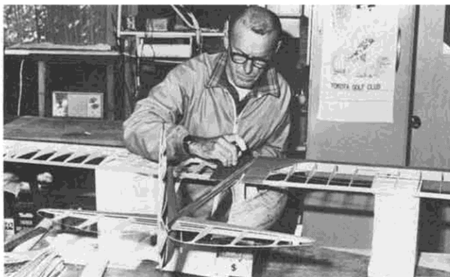
Test fitting the basic structure. The tail boom is made from a one inch diameter aluminum tube towel rack.
