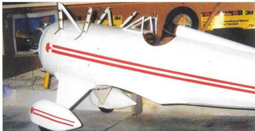
The fuselage with wings and cowl removed shows the cabane struts arrangement and fuel line detail.
