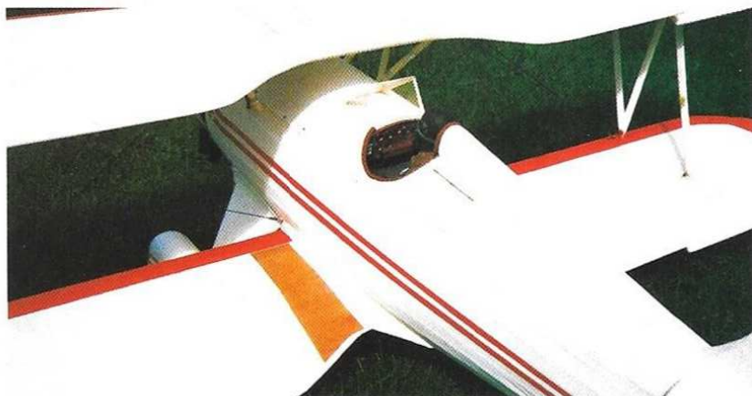
Rear three-quarters view shows the cockpit, luggage locker, centre section fuel tank and wing walk detail which breaks up the outline of the Waco and brings the model to life.
