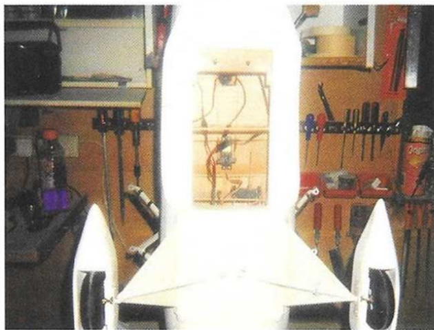
No problem with fitting the radio gear in that cavernous fuselage opening.
