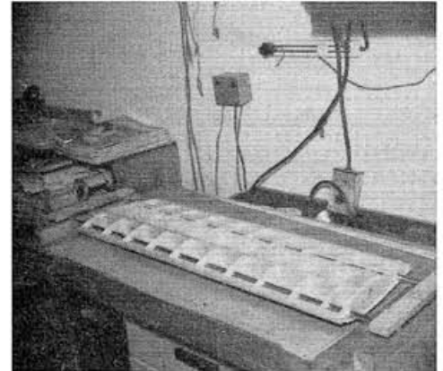
Below, Left: The panel complete, pin holds filled, completely finish sanded and ready for removal from the jig. Below: Panels pinned at the desired dihedral angle. Install tip blocks, fiber glass the center section and your wing is ready for monocoque or your favorite finish.
