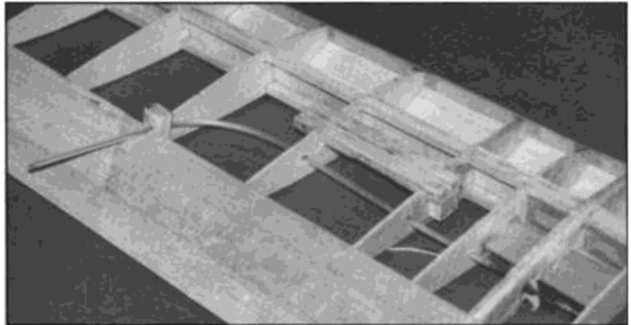
Hardwood block with notch holds the Du-Bro flex cable in place during assembly of aileron pushrod cable.
