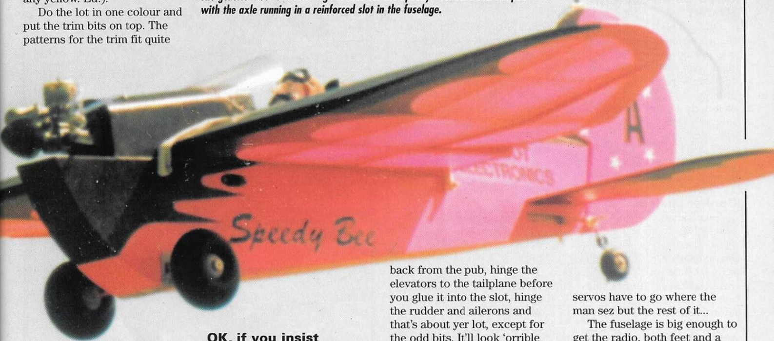
The generic 'Bee' undercarriage is used for the Speedy - rubber band damped with the axle running in a reinforced slot in the fuselage.
