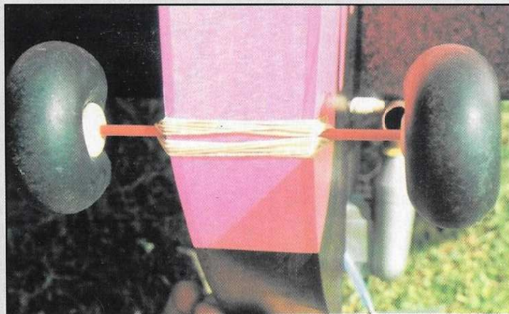
The generic 'Bee' undercarriage is used for the Speedy - rubber band damped with the axle running in a reinforced slot in the fuselage.
